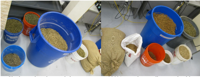
Clockwise from bottom left are straw pellets with 1% kaolin, grass with 25% camelina seed, 100% grass, 50/50 grass/camelina meal in the white pale, 100% straw in the large barrel, and 100% grass in the burlap
