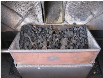
Burn pot of the Model 6041 US Stove Multi-Fuel Heater after burning 9.8 lbs of straw pellets. The stove stayed lit, but it would likely have gone out soon either to an overfull burn pot or a stalled agitator.
