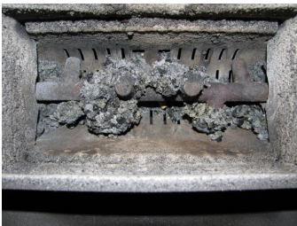
Burn pot of the Model 6041 US Stove Multi-Fuel Heater after burning 9.8 lbs of straw pellets. The stove stayed lit, but it would likely have gone out soon either to an overfull burn pot or a stalled agitator.
