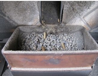
Burn pot of the Model 6041 US Stove Multi-Fuel Heater after 17.06 lbs of straw pellets with 2% CaCO 3 . Still a lot of ash, but the grains are smaller and the agitator was not grinding on them.
